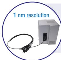
Fiber-coupled multi-spectra system with 8 to 32 channel simultaneous measurements
