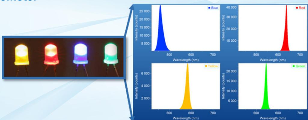
PoliSpectra Quad Spectrometer is capable of simultaneously measuring 4 channels of 1024 pixels spectra. The picture above shows the emission spectra of 4 different color LEDs measured using Ø 200 µm core fibers.
