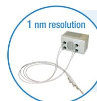
CCD spectrometer for simultaneous acquisition from 4 fiber inputs (470-730 nm)
