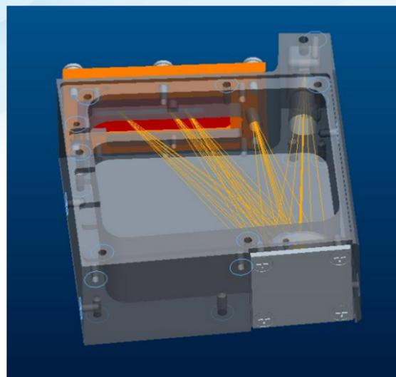
Concave-grating mini spectrometer optical mechanical design.
