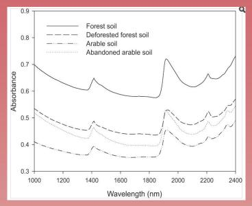
The exclusive DARWin SP Data Acquisition software included with each unit allows for full featured instrument control and data handling. The LF-2500 can be used as a lab system or in the field with an optional battery. In field studies, the LF-2500 can provide critical information on different soil characteristics, for example in the spectra at left, distinguishing between arable soil in use, arable soil not in use, forest soil, and de-forested soil.
