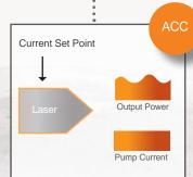
ACC (Automatic Current Control) mode is standard for all devices. The laser is controlled from diodes current set point.
