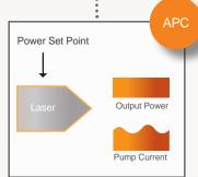
APC (Automatic Power Control) mode allows to control the laser at a fixed output power set point. The device maintains a constant optical output power monitored with a photodiode. The current is adjusted automatically.
