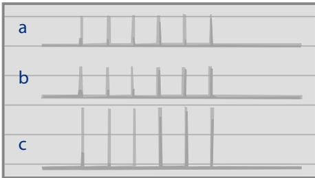
Two laser output synchronized to double the pulse energy and peak power,
