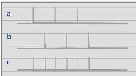
Two laser output combined with an adjustable delay to double the pulse repetition rate,
