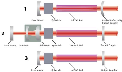
**3 Stable Resonator Option - 50Hz to 200Hz**
