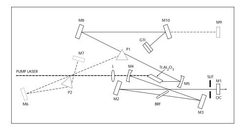
Nearly transform-limited picosecond pulses are generated by Coherent's patented Kerr Lens Modelocking (KLM) process in the picosecond cavity version of the Mira® 900-P Titanium:Sapphire Laser. The required intracavity Group Velocity Dispersion (GVD) for picosecond pulses is generated by a Gires-Tournois Interferometer end-mirror in the cavity. In the Mira 900-P, the intracavity GVD is automatically adjusted to the correct
