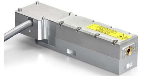
For generating high peak power IR pulses of a few hundred picoseconds, microchip lasers are economical, compact, and extremely reliable. Sub-nanosecond 1064nm pulses are indeed directly generated from the diode pumped passively Q-switched Nd:YAG microchip engine.
