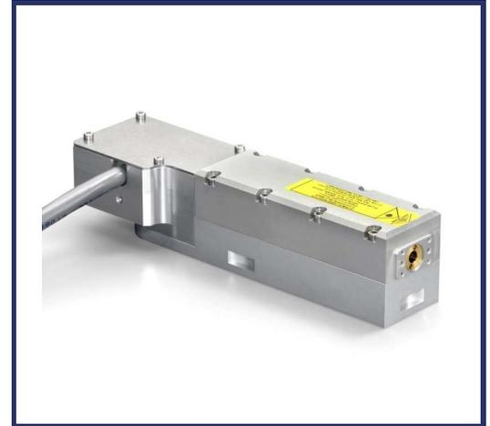
For generating high peak power IR pulses of a few hundred picoseconds, microchip lasers are economical, compact, and reliable. Sub-nanosecond 1064nm pulses are indeed directly generated from the diode pumped passively Q-switched Nd:YAG microchip engine.
