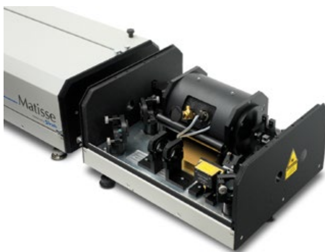
Matisse 2 TX with separate high-finesse reference cavity with Pound-Drever-Hall feedback scheme.
