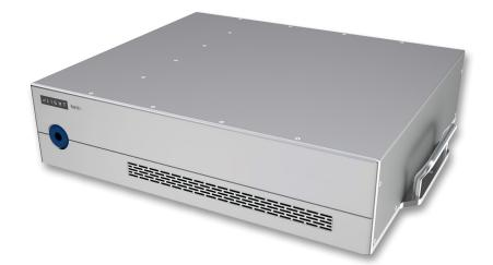
nLIGHT's helix<sup>™</sup> picosecond fiber laser is the industry's first cost-effective solution for highprecision micro-materials processing. Designed to meet the highest quality and reliability standards for maintenance-free 24/7 industrial operation, the aircooled system provides a near-diffraction-limited, highpeak-power, short pulsed beam at 1064 nm. The small footprint of the laser head coupled with an intuitive user interface allows for ease of integration into any laser machine tool.
