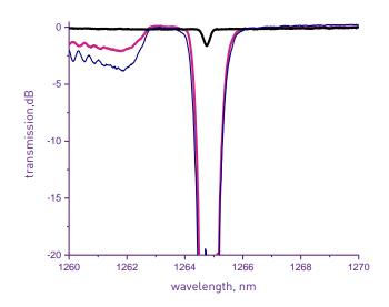
0.7nm. Output grating with reflectivity 5% - 40% has FWHM 0.15  $\div$  0.35nm. Mismatching LR grating relative to HR one is up to  $\pm$  0.1nm. For fiber lasers with narrow line we are presented FBG pairs with FWHM around or less 0.1nm with ideal matching without adjustment. The transmission spectrum of FBGs Pair for Yb laser and Raman converter are presented in the graph.
