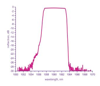
gain flattening EDFA and ASE light sources, band stop filters, in ultrafast mode – locked fiber lasers, powerful laser and chromatic dispersion compensation telecom systems. The optical spectrum of high reflection Chirped FBG for powerful fiber laser is presented in the graph.
