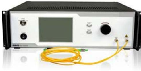
Techwin 2.0 $\mu$ m CW fiber lasers are eye-safe high power fiber lasers. These fiber lasers employ integrated design of all fiber structure and use double cladding fiber pumping technology, thus realizing high performance output laser. The output power can be up to 20W and near diffraction-limited beam quality is achieved at the same time. They can be widely used in the areas of scientific research, experimental teaching and device testing.
