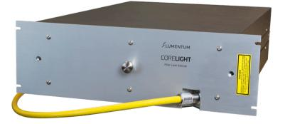
CORELIGHT Series fiber laser modules are compact ytterbium fiber lasers that offer straightforward integration into new and existing manufacturing tools and use a customer's existing power and control system for cost efficiency. Module control and monitoring are accomplished through analog and Ethernet communication ports. Multiple, user-accessible, real-time system logs assure detailed operational history is available for review at any time.
