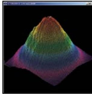
THz laser beam at 1.6THz (184 $\mu$ m).
