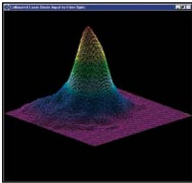
CO<sub>2</sub> laser with cavity misalignment.
