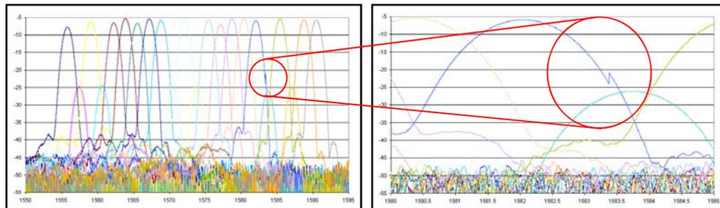
dBm Optics uses a patented technique to rapidly determine the correct measurement range, change to that gain, forcibly inject or deplete charge from the amplifiers (to force rapid settling), then make the measurement. All this (including the measurement) takes less than 10  $\mu$ s. Our intra-range linearity is assured using a special calibration technique that occurs in the background.
