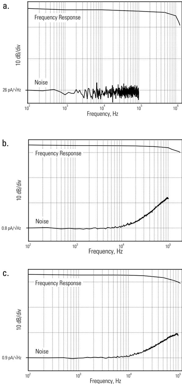
For the Model 232 the bandwidth is 900 kHz for the low gain setting and 150 kHz for the medium and high gain settings.
