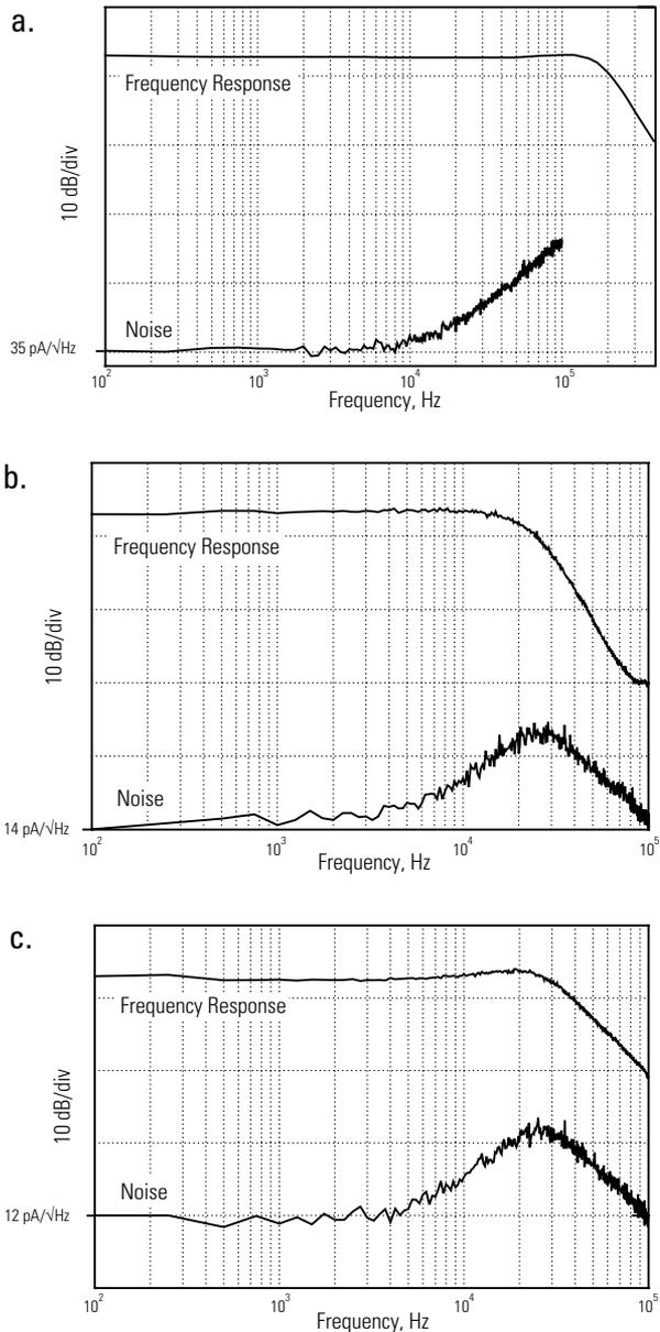
For the Model 2034 the bandwidth is 700 kHz for the low gain setting, 90 kHz for the medium gain setting, and 80 kHz for the high gain setting.
