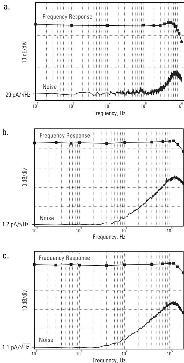
For the Model 2033 the bandwidth is 200 kHz for the low gain setting, 30 kHz for the medium gain setting, and 30 kHz for the high gain setting.
