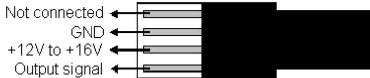
FIG. 1-4 MOLEX CONNECTOR PIN-OUT IN MT VERSION
