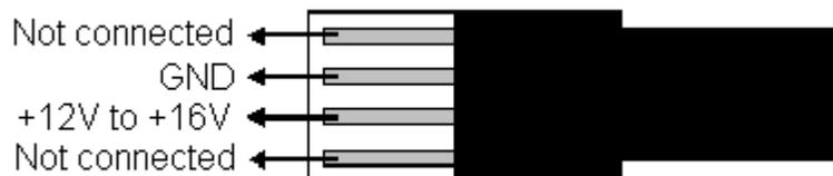
FIG. 1-6 MOLEX CONNECTOR PIN-OUT IN BT VERSION
