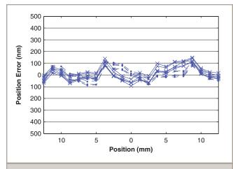
ANT95XY-025-PLUS accuracy and repeatability, five runs, bi-directional for the X (lower) axis. The total accuracy of 240 nm over 25 mm travel is significantly better than other offerings and half of its stated specification.
