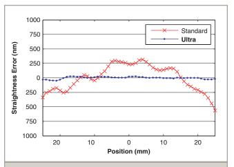
ANT95XY-025 straightness error comparison between the BASE and ULTRA models shows a dramatic improvement in this specification.
