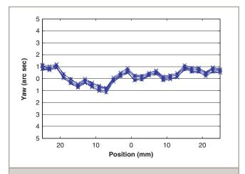
ANT95XY-050-PLUS Y (upper) axis yaw, five runs, bi-directional. Highly repeatable, lowest angular error over full travel.
