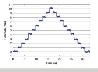
ANT95XY-025-PLUS lower axis 1 nm step plot. Best-in-class resolution and exceptional in-position stability for large travel stages.
