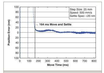
ANT95XY-025-PLUS step and settle performance at full travel and 1 kg payload for the X (lower) axis. Industry-best settling times significantly improve throughput for most applications.
