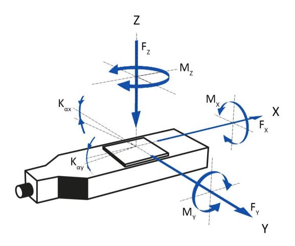
Direction of the axes and torques for linear stages, dimensions in mm
