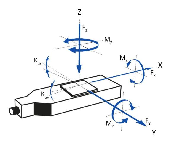
Direction of the axes and moments for linear stages
