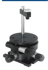
The model 860-0110 tilt/rotation stage provides two independent tilt adjustments within  $\pm 5^{\circ}$  range and  $\pm 4^{\circ}$  in-plane rotation adjustment. Precision screws provide 9 arcsec resolution in rotation and both tilt planes (adjustment screws M6×0.25, 3 pcs.).
