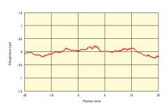
XM stages deliver ripple-free motion as required by many precision scanning and wafer inspection processes. Shown is the straightness of an XMS50 during one forward and return cycle, measured with an interferometer.
