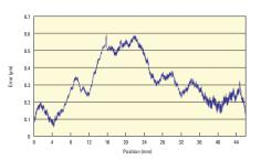
Accuracy of a XMS50 stage after linear error correction. The data was taken dynamically at a rate of 10 kHz while the stage was moving at a speed of 100 mm/s. Both the encoder and the interferometer positions were acquired by an XPS motion controller with a latency of less than 50 ns between the different signals
