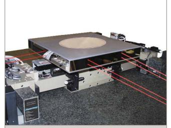
Multi-axis interferometer feedback is available to control X and Y position, as well as Y-axis yaw. Use of a remote detector allows one laser source to be used for multiple axes.
