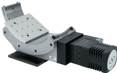
**Note:** To access the interface holes of the carriage, simply move the bottom stage to its extreme position. Two c'bores will be accessible from one end of travel and the other two holes will be accessible from the other end of travel. For example, between the BGM160 and BGM200, use the M6 holes in a 6.14 x 3.62 (156 x 92 mm) pattern. BGS80 on BGM120, use M4 holes in a SQR 1.89 (48 mm) pattern.
