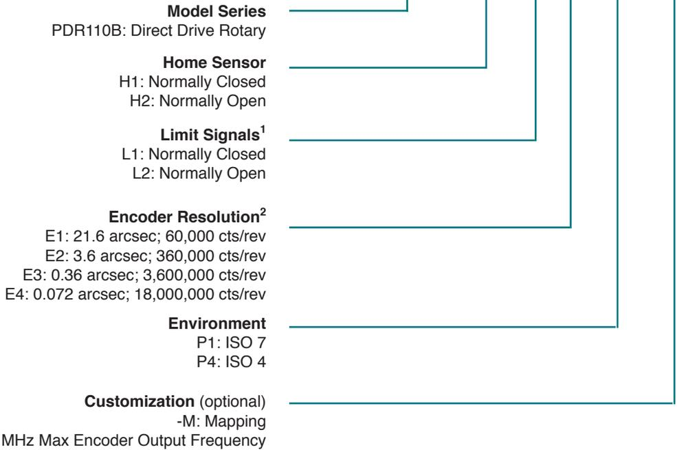
Notes: 1) The PDR series does not include limit sensors. The Limit Signal options are provided for compatibility with motion controller requirements. 2) Standard encoder max output frequency is 12.5 MHz.
