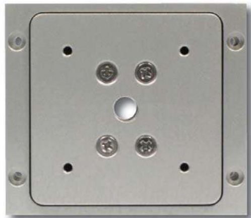
Nano-MZ (actual size) constructed from aluminum.
