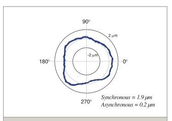
ANT95R radial error plot illustrating outstanding synchronous and asynchronous error motion performance.
