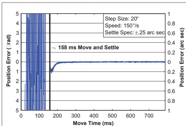
ANT20G-090 step and settle performance. Outstanding settling time enhances throughput of most applications.
