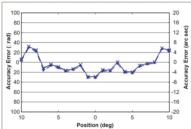
ANT20G-090 accuracy, five runs, bi-directional, uncalibrated, shows the high level of system accuracy.
