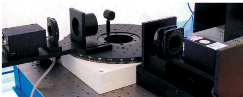
Scattering Photometer Experiment Setup using MRSC Series rotation stage
