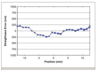
ANT95L-025PLUS straightness error, five runs, bi-directional. Exceptional and highly repeatable – five times more accurate than the stated specification.
