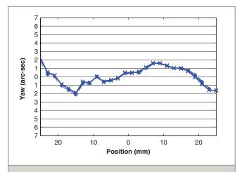
ANT95L-050PLUS yaw, five runs, bi-directional. Highly repeatable, minimal yaw error enhances system positioning accuracy.
