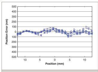
ANT95L-025PLUS accuracy and repeatability. This multiple test run over an extended period of time shows the high level of system accuracy and repeatability.
