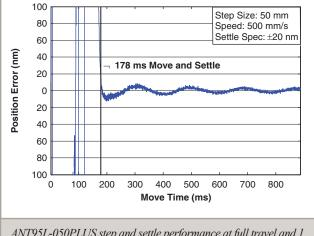
ANT95L-050PLUS step and settle performance at full travel and 1 kg payload. Outstanding settling time enhances throughput of most applications.
