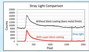
Stray light comparison between uncoated and coated cavity (Super Black) measured by far field illumination using tungsten lamp – zero order
