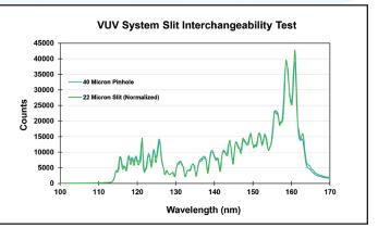
VUV system slit interchangeability test with 40  $\mu m$  pinhole and 22  $\mu m$  slit
