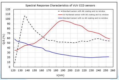
UV hardened sensor provides increased lifetime, however no warranty is provided on any sensor exposed to VUV.
