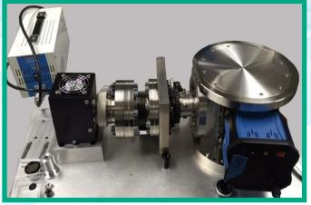
N<sub>2</sub>-purged set-up shown with Hamamatsu: L10366 VUV light source
