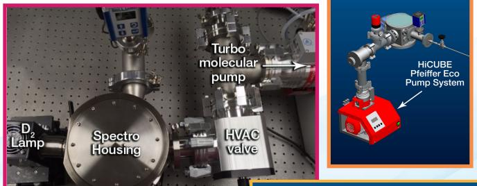
Config #2: Nitrogen-purged CCD temp: -25° C
