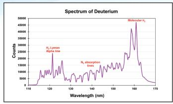
Spectrum of deuterium lamp shows enhanced sensitivity starting from 113 nm with 22 µm slit (0.45 nm resolution)
