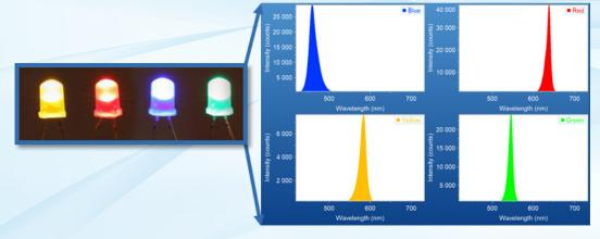
PoliSpectra Quad Spectrometer is capable of simultaneously measuring 4 channels of 1024 pixels spectra. The picture above shows the emission spectra of 4 different color LEDs measured using  $\emptyset$  200  $\mu$ m core fibers.
