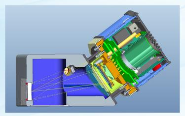
CiCi-Raman-NIR strudy optical housing with TE-cooled Syncerity CCD detector.
