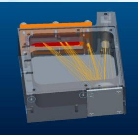
Concave-grating mini spectrometer optical mechanical design.
