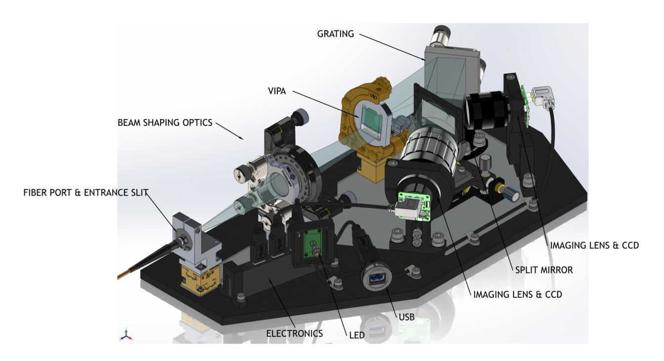
Light enters the HyperFine Spectrometer through a fiber. A VIPA etalon, manufactured using LightMachinery's proprietary fluid jet polishing technology, is used to produce very high dispersion in the vertical axis with sub picometer resolution. This is followed by a conventional grating to disperse overlapping orders in the horizontal direction and produce a 2D spectrum of the input light.
