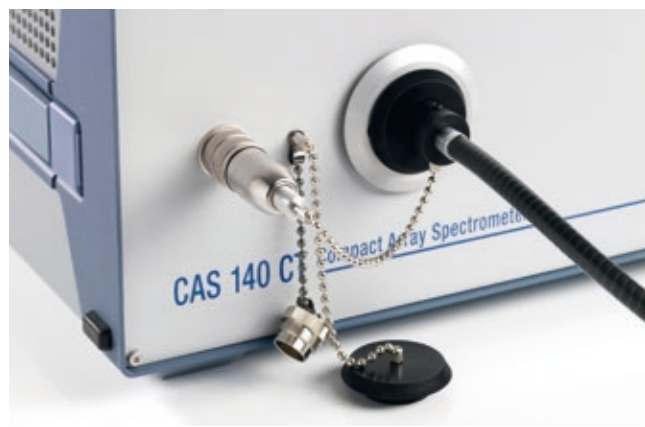
The Ident key identifies measurement adapters
