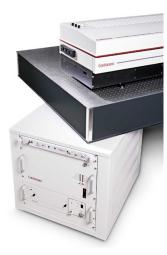
rack mounted to simplify maintenance and service. It uses distributed intelligence, with microprocessors in both the laser head and power supply. Communications from the head to the supply are digital and much more reliable than TTL and analog inputs.
