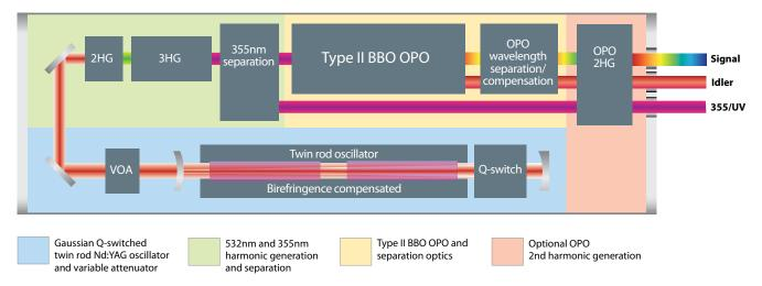
Schematic shows the compact arrangement of the combined pump laser and Aurora II Integra OPO in a single housing.
