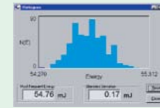
Distribution of the output energy per pulse for 500 consecutive shots. Range of histogram \pm 1\% of mean value. Standard deviation \sim 0.3\% .
