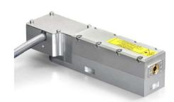
For generating high peak power IR pulses of a few hundred picoseconds, microchip lasers are economical, compact, and extremely reliable. Sub-nanosecond 1064nm pulses are indeed directly generated from the diode pumped passively Q-switched Nd:YAG microchip engine.
