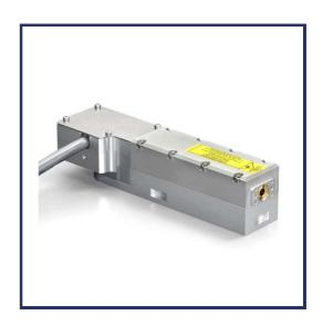
For generating high peak power pulses of a few hundred picoseconds, microchip lasers are economical, compact, and reliable. Visible and UV wavelength are generated from the harmonic conversion of an IR passively Q-switched Nd:YAG microchip engine, within a sealed package ensuring incredibly long lifetime even in harsh industrial environment.
