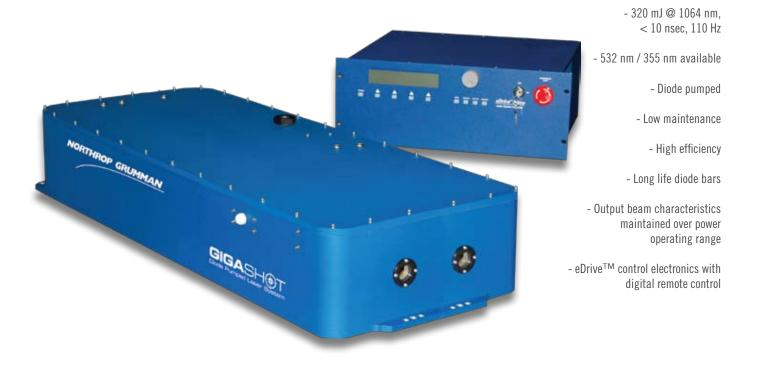
The Gigashot laser system is a new diode-pumped solid–state (DPSS) Nd:YAG laser that delivers 320 mJ per pulse at 1064 nm at a repetition rate of 110 Hz. An unstable laser resonator with two polarization compensated QCW pumped DPSS modules delivers a low divergence output beam with high spatial uniformity. The birefringence compensation between the pump modules eliminates any low order depolarization losses and ensures excellent beam quality even at high frequencies and high average power.
