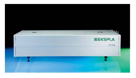
PL11M series picosecond mode-locked diode pumped laser offers 1 W output power at 1064 nm. It features high 1 MHz repetition rate, short 10 ps pulse duration and excellent beam quality (M² < 1.5).
