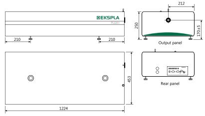
Fig 2. Dimensions of PL2250 series laser head
