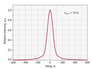
Typical autocorrelation curve of FF1000 laser
