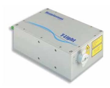
The T-Light is a robust and compact turn-key femtosecond fiber laser. It offers exceptional performance for a variety of applications, from ultrafast spectroscopy to THz physics. The laser design is based on polarization (PM) maintaining fiber components, which is the key to stable operation. Menlo Systems' unique figure 9® mode locking technology ensures reproducible and long-term stable operation. The result is a reliable fiber laser source, designed for 24/7 operation.
